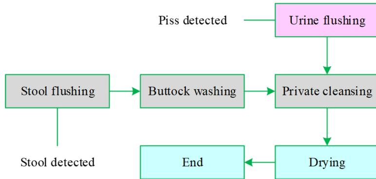
**Figure 3.** Work flow of defecation function in automatic mode.
