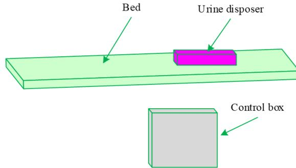
**Figure 5.** Schematic diagram of the location of the urinal processor and control box.
