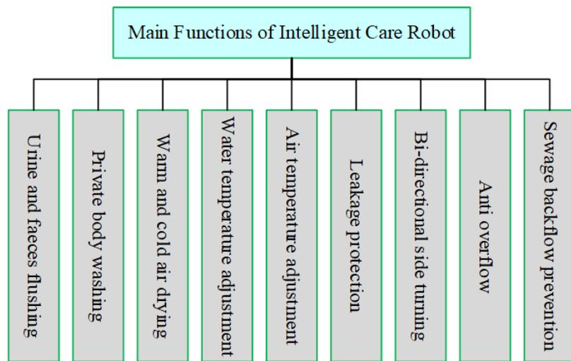
**Figure 2.** The main function box of intelligent care robot.
