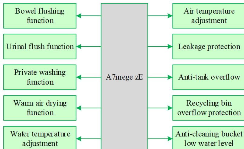
**Figure 6.** Functional block diagram of the control system.
