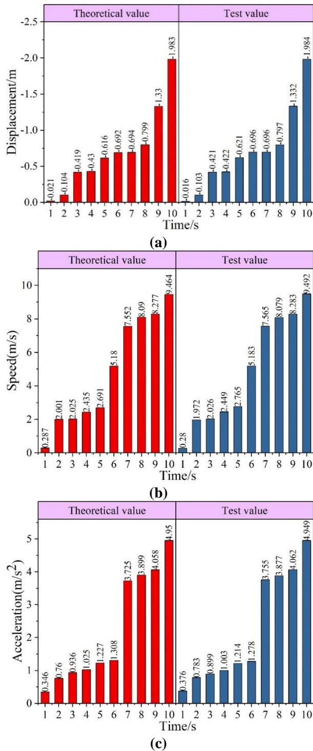
**Figure 7.** Vertical dimension verification analysis results (a) displacement; (b) speed; (c) acceleration.
