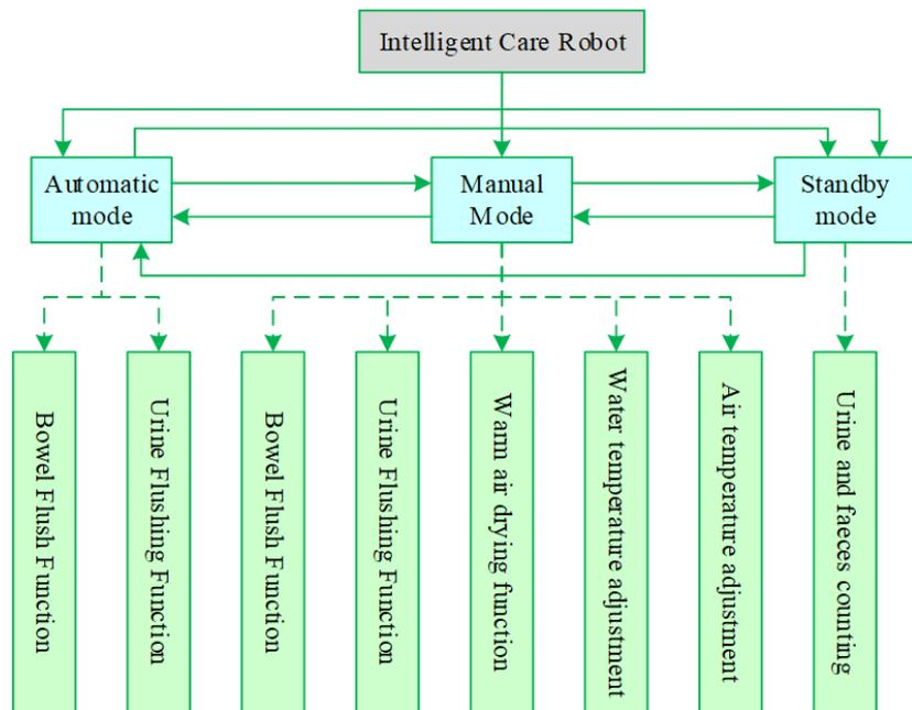
**Figure 4.** Diagram of patterns and functions.
