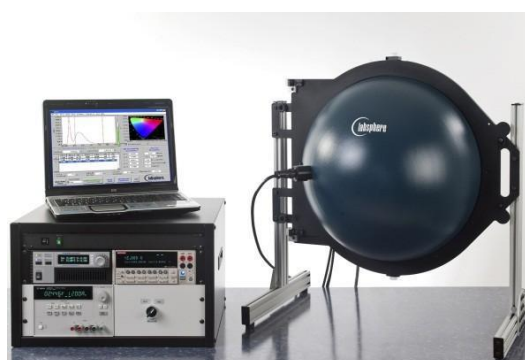
Figure 6. Integrating sphere test experiment.
