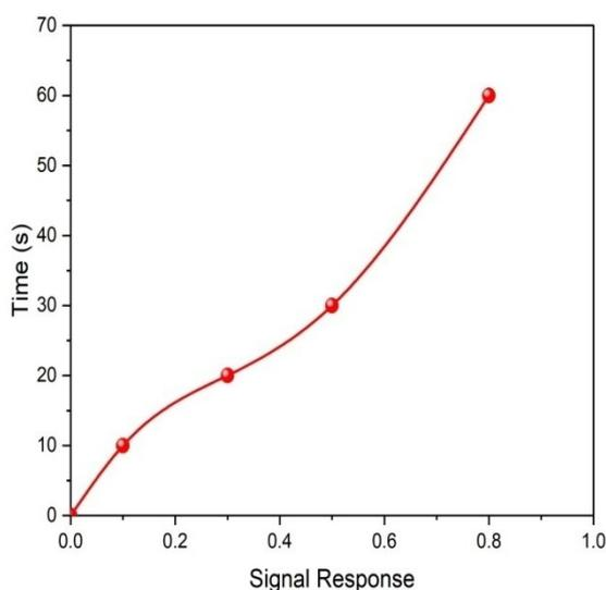
**Figure 6.** Signal response of the biosensor to the target analyzed as a time response curve.
