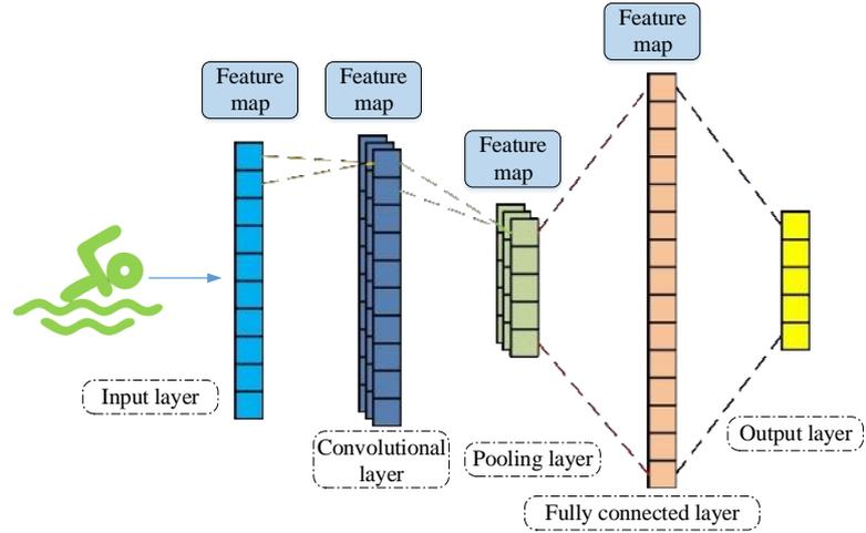
**Figure 2.** CNN architecture.
