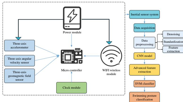
**Figure 3.** Swimming posture recognition model based on inertial sensors and CNN-SVM.
