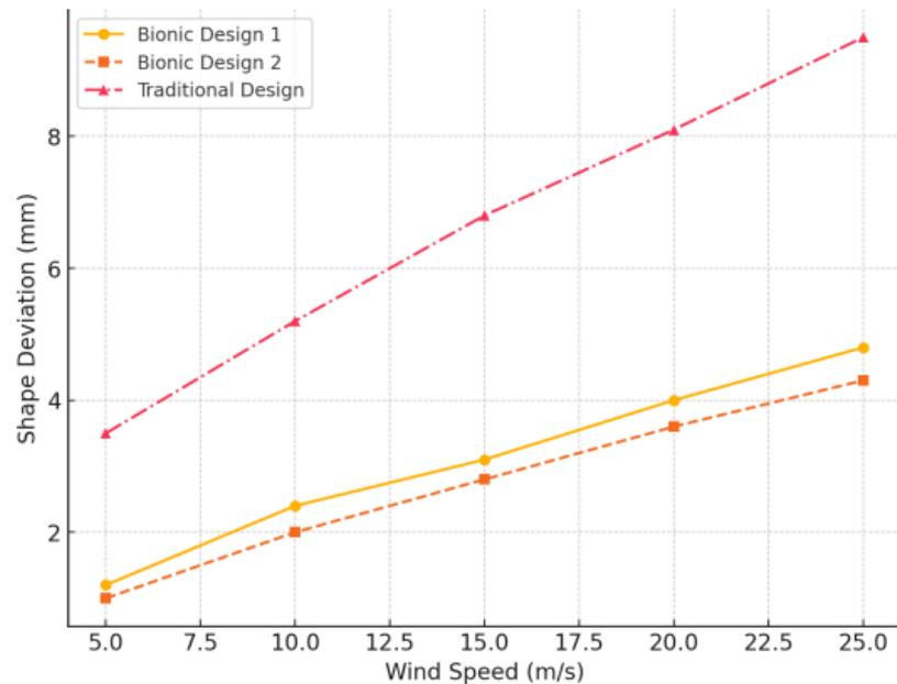
**Figure 1.** Morphological shift trend of different bionic wave structures under wind speed variation.
