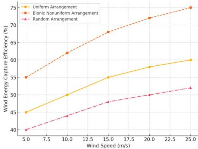
**Figure 2.** Simulation results of wind energy capture efficiency with different blade arrangements.
