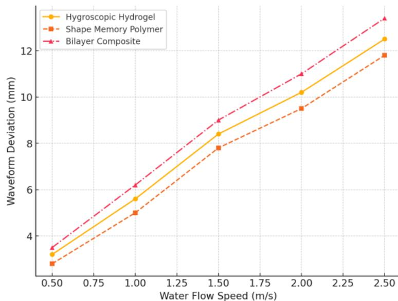
**Figure 7.** Trend of wave patterns of flexible mechanisms under different water flow rates.
