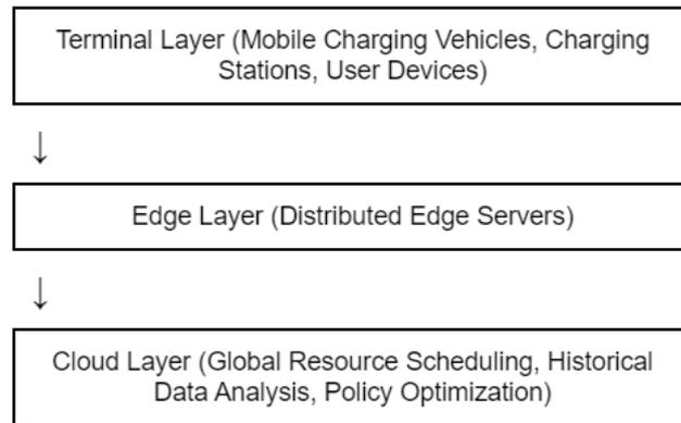
**Figure 3.** Schematic diagram of edge computing architecture.
