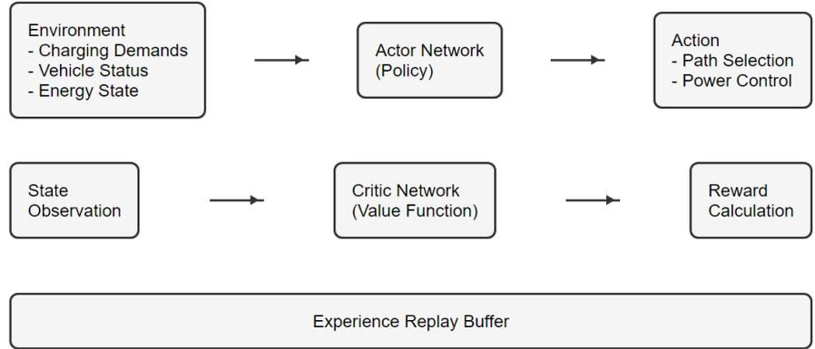
**Figure 4.** Framework diagram of real-time scheduling algorithm.
