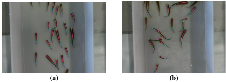
Figure 13. Error analysis diagram of fry size measurement. (a) Fish body curvature error diagram; (b) Fish body occlusion error diagram.
