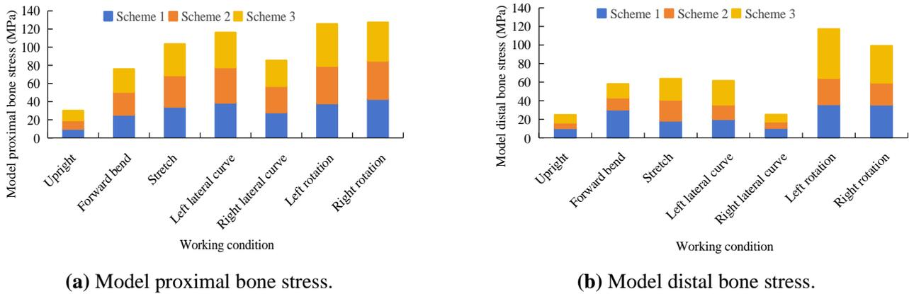
**Figure 3.** Proximal and distal stress analysis.
