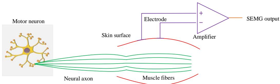
**Figure 1.** Principle of surface electromyography signal acquisition in target muscle area.
