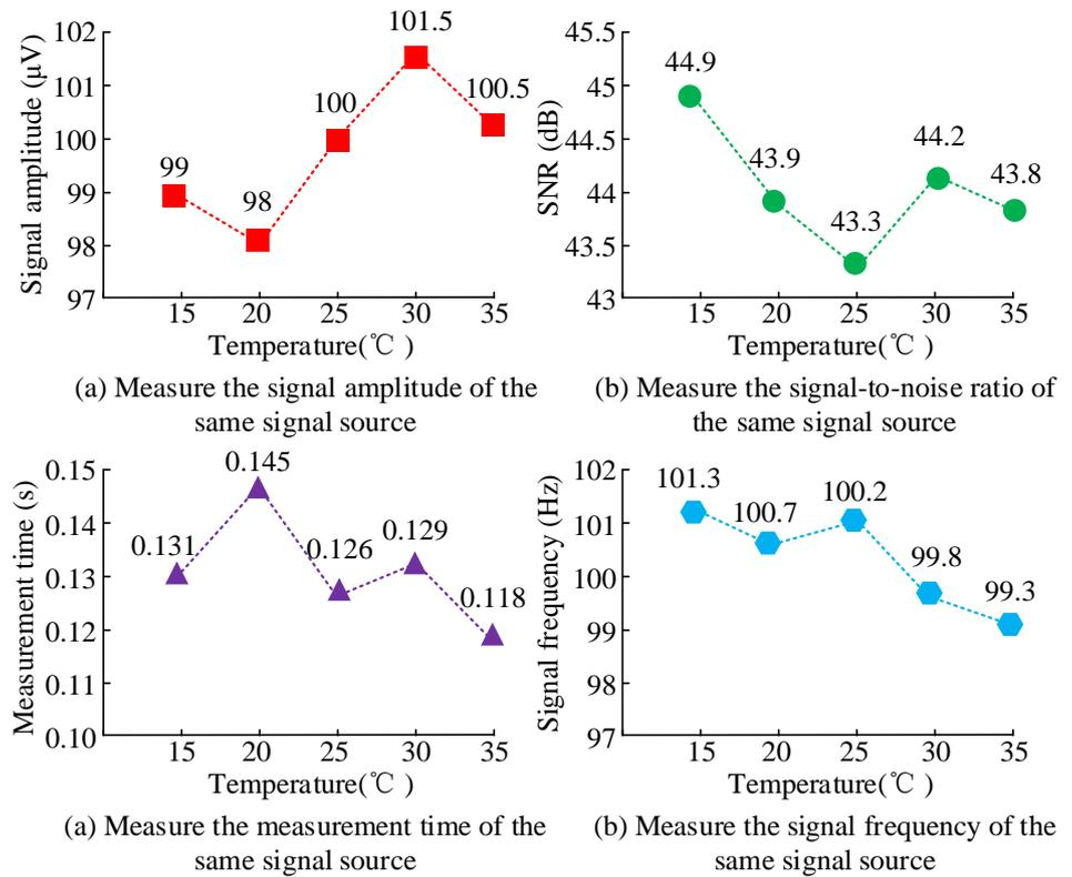
**Figure 5.** Stability of surface electromyography signal acquisition.
