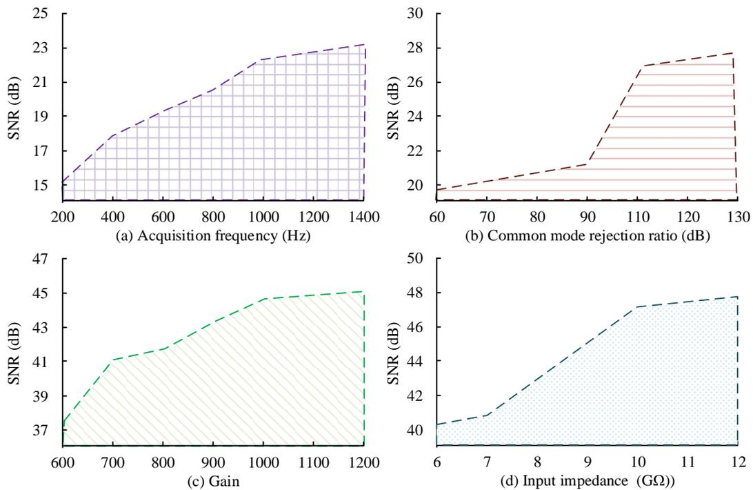
**Figure 3.** Optimization of key parameters for surface electromyography.
